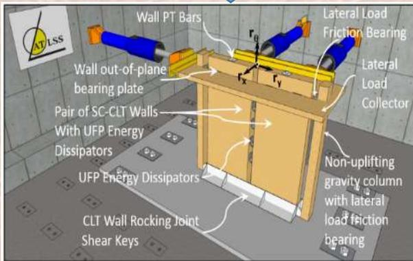
Components testing at NHERI@Lehigh Structural Lab (expected 2017)
